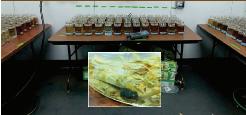
Tadpole experiment setup at SUNY-ESF. Each quart jar contains 0.8 grams of dried leaves and one wood frog tadpole. Inset: healthy tadpole in a jar with crushed chestnut leaves.
