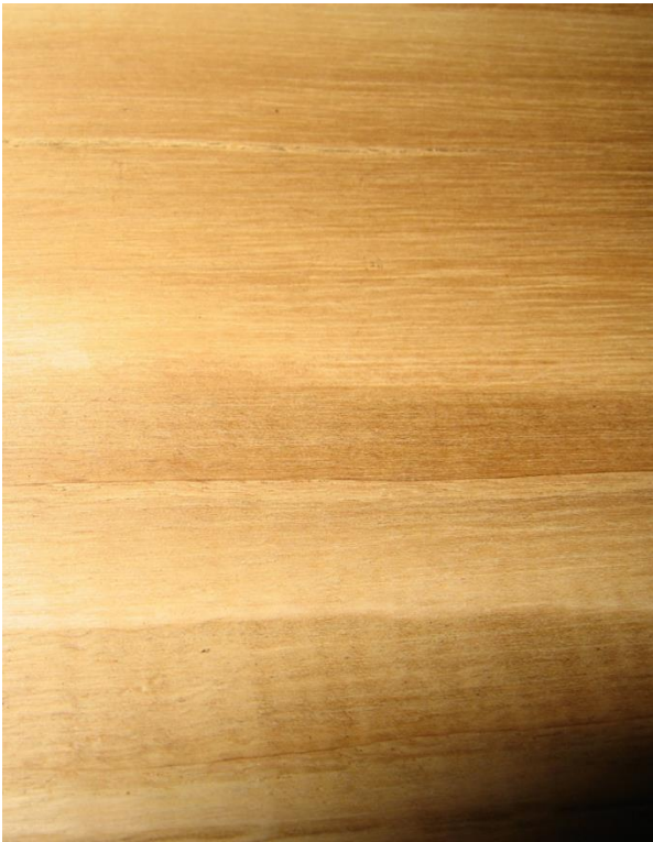
Figure 3. Face grain of Chinese chestnut wood. Notice the less pronounced earlywood and slightly different color.
