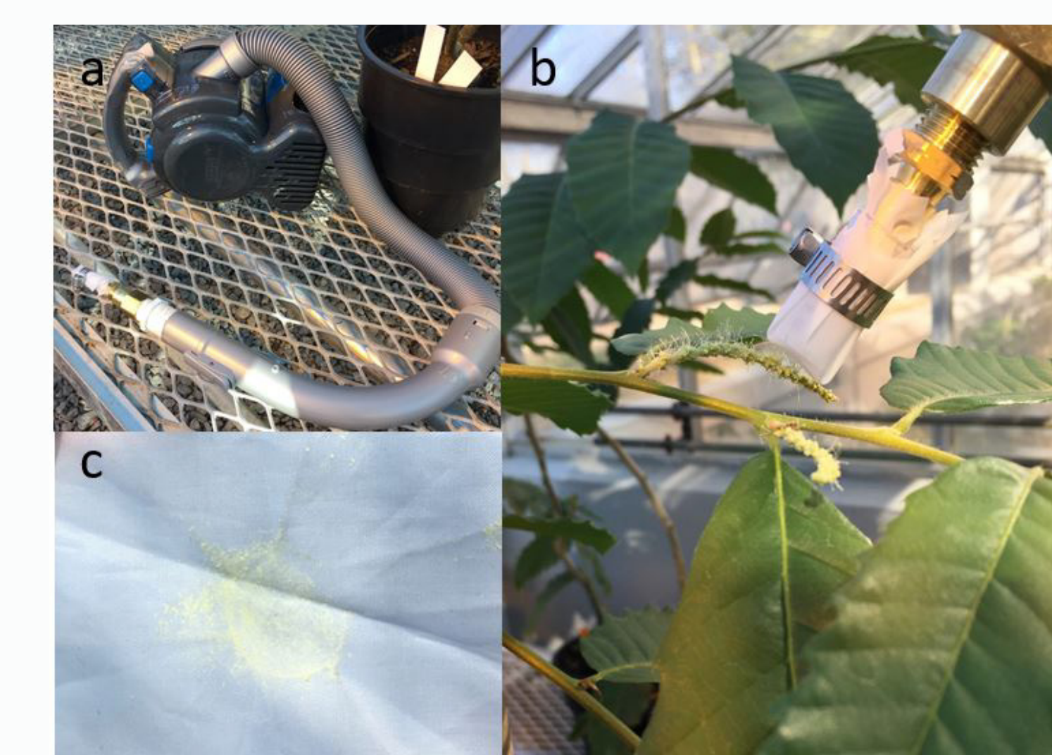
Fig 7. A) Cordless Black & Decker vacuum. B) Modified nozzle to filter debris and trap pollen. C) Pollen grains collected on mesh in cluster.
